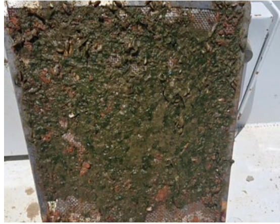
Pegasus Loop Line Cla-Val Strainer Screen
